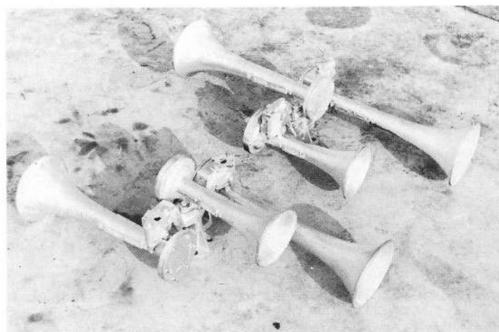
Nathan P3R2's: (left) IC, SR, SP SW1500's (note holes--missing blanking caps); (right) SP road power, NP.
