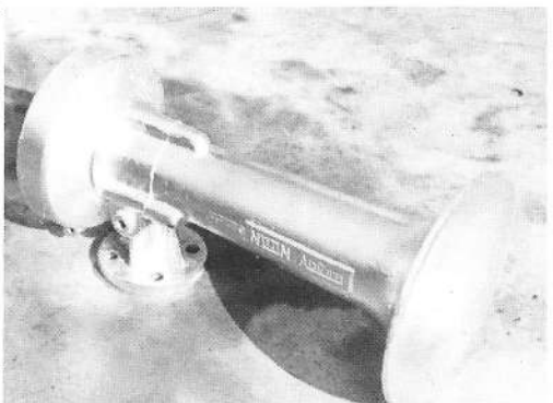
Nathan MS1 using single base and #1 bell, common on many switchers and early Geeps.
